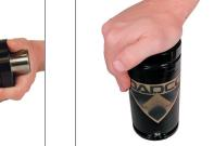
4S. After all of the gas pressure is exhausted, be sure that the piston rod will freely retract into the tube manually. If not, try depressing the valve again. It still unsuccessful stop and contact DADCO.
