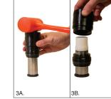
vertically tap the Assembly Cap Cartridge Starter Kit (90.335.x) to drive the cartridge down the rod. Be careful not to force the cartridge at an angle as the Cone or rod, making sure that seal could become damaged.
