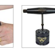
Cartridge Assembly select the proper common rod end M10) and thread the T-Handle (90.320.M) into the rod end while pulling out the assembly.
