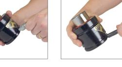
2. To decrease the gas spring pressure, depress the valve stem using a DADCO Valve Bleed Tool, (90.360.4), or a DADCO Pressure Analyzer, (90.315.5).
