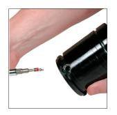
3S. Thread a new Compact 1L. Check the port for deposits Valve, (90.260), or Cartridge or burrs and clean thoroughly. Valve (90.265), into the port Inspect the service fitting and until it fits snugly on the seat. replace if it shows signs of Avoid over torquing the valve. damage. Lubricate threads and seals on the fitting and thread the service fitting into the gas
