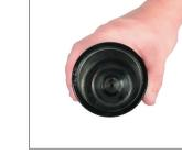
3. Inspect the Tube Assembly for any damage, especially around the mouth of the Tube Assembly. Lightly polish out any scratches at the mouth of the Tube Assembly to avoid damaging seals during the reassembly process. If damage to the Tube Assembly is severe it must be replaced Wash, clean and dry the inside thoroughly.
