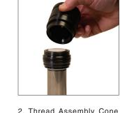
2. Thread Assembly Cone (90.331.x) from Cartridge Starter Kit (90.335.x) onto rod. Slide Cartridge Assembly making sure that the wiper end marked "TOP" is facing up. Place Cartridge Assembly Cap (90.330.x) from Cartridge Starter Kit (90.335.x) on top of Cartridge Assembly.
