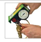
Attach Charging Assembly (90.310.040) to the quick disconnect filler valve on the
