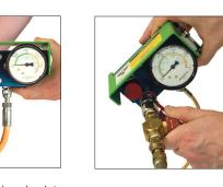
2L. Attach Charging Assembly (90.310.040) to the quick disconnect filler valve on the control panel.
