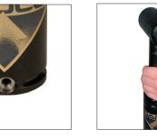
Stand the gas spring upright. Place a removal sleeve, (90.340.x), longer than the stroke over the rod. Tap the sleeve until the Dust Cover, (90.246.U.x), is loosened. Remove the Dust Cover and
