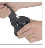
tool is firmly seated below the c-ring, begin pushing it toward the outside of the gas spring service thread (M6, M8 or the rod and discard. Retain the can. The handles will close naturally, and the c-ring will be extracted as you complete
