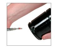
3S. Thread a new Compact Valve, (90.260), or Cartridge Valve (90.265), into the port until it fits snugly on the seat. Avoid over torquing the valve.
