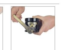
3L. Unthread the service fitting and wipe with a clean cloth. Proceed to "II. Port Maintenance" Linked Mode
