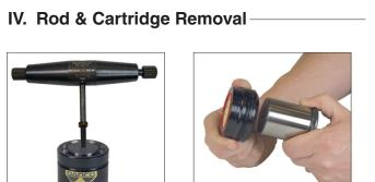
4. Once the hooked end of the 1. To remove the Rod and 2. Once the cartridge and rod are removed from the Tube Assembly slide the cartridge off rod for inspection and reuse.
