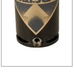
1L. Check the port for deposits or burrs and clean thoroughly. Inspect the service fitting and replace if it shows signs of damage. Lubricate threads and seals on the fitting and thread the service fitting into the gas spring port.
