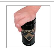
2L. Verify that all pressure is 3L. Unthread the service fitting relieved by manually retracting and wipe with a clean cloth. the piston rod into the tube. If Proceed to "II. Port the rod will not fully retract Maintenance" Linked Mode release the remaining step 1L. pressure. If still unsuccessful stop and contact DADCO.
