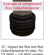
UX.6600 - UX.9600 models with stroke lengths 150 mm and above, the collar/dampener is black and looks like a series of loops. If there are any splits. cracks or excessive wear then the collar needs to be replaced. To verify the condition, measure the Rod Collar/Dampener height and refer to the chart for the A measurement. If the height is out of tolerance Contact DADCO for repair or replacement. If only the wear band is damaged, it may be
