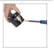
Valve, (90.260), or Cartridge Valve, (90.265), by unscrewing is leaking pressure or sticking it with the Port Servicing Tool, (90.320.8).
