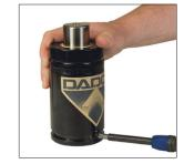
2S. Remove the Compact Valve, (90.260), or Cartridge Valve, (90.265), by unscrewing it with the Port Servicing Tool, (90.320.8).
