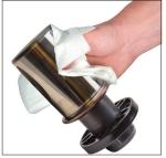
2. Lightly polish the rod surface with an emery cloth (600 grit). Inspect the finish of the rod for any scratches or gouges. If the rod is damaged it must be
