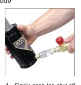
3. Open the main valve on the nitrogen tank. Set the desired charging pressure on the regulator. Do not exceed the maximum charging pressure
