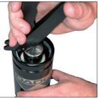
3. Remove the C-style Retaining Ring, (90.285.x.), using a C-Ring Removal Tool, (90.356 or 90.355). Position the hooked end of the tool below the c-ring. For best results locate the tool nea either end of the c-ring.
