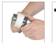
1. Lightly polish the rod surface 2. Inspect the Tube Assembly with an emery cloth (600 grit). for any damage, especially Inspect the finish of the rod for around the mouth of the Tube any scratches or gouges. If the Assembly. Lightly polish out rod is damaged it must be any scratches at the mouth replaced. of the Tube Assembly to avoid damaging seals during the reassembly process. If
