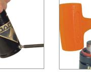
9. Install the new Dust Cover, (90.246.U.x). Tap with a soft mallet until the top of the Dust Cover rests flush with the top of the can. The rod wiper should
