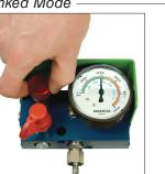
Verify that all pressure is relieved by manually retracting the piston rod into the tube. If the rod will not fully retract release the remaining pressure. If still unsuccessful
